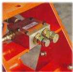
**4**)Built-in priority valve system monitors the oil flow, providing the correct volume to obtain maximum performance by the compaction plate and avoiding damage to the hydraulic motor due to excessive flow.
