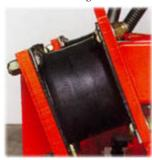
1)Rubber vibration mounts are angled to the base, so that the pressure exerted by the boom on the top plate causes the mounts to convert from a shear to a compression mode (Patented System).
