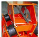
2)The hydraulic motor and hoses are positioned within the protective cradle to prevent them being snagged or damaged on trench walls.
