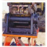
**3**)Engineered for easy, direct attachment to existing hydraulic hammer mounting heads. This time saving system is ideal for use with quick hitch arrangements. A multi setting, 360° swivel head attachment is also available.
